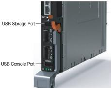
Use the lower USB console port (Figure 1-3) to manage the switch through an RS-232 serial interface. This port provides a direct connection to the switch and allows you to access the command-line interface (CLI) from a console terminal connected to the port through the provided serial cable (with USB type-A to female DB-9 connectors).
