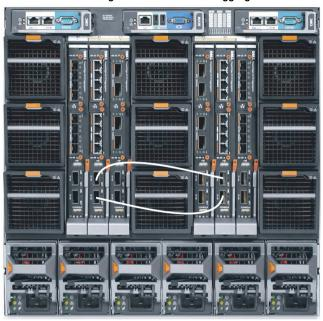
Figure 1-9. Switch Stack Using 40GbE Ports on Two Aggregators
